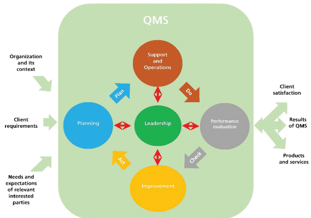
Figure 1. Structure of plan–do–check–act cycle in ISO 9001:2015.2 Abbreviation used: QMS, quality management system.
